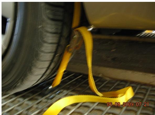
Example of hook being blocked by tire.
